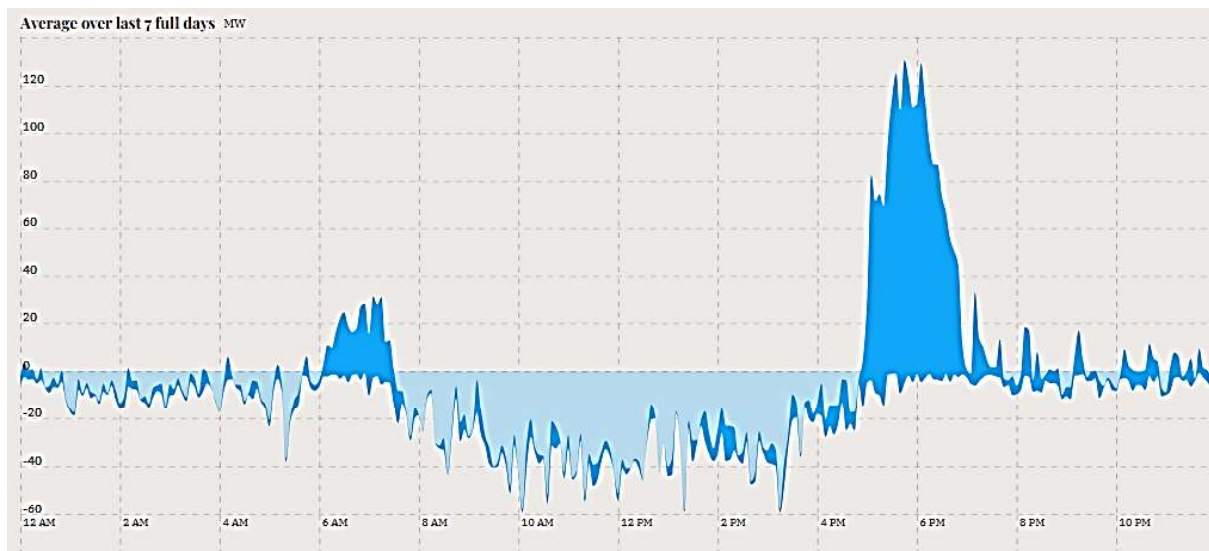
Figure 7-6. Time of day operations for BESS' in NSW (7 day average, 26 April 2024)
